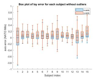
Figure 13: Box plot of x and y-axis lay errors for 15 subjects, with outliers removed for ease of reading.
