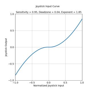
Figure 4: A graphical representation of the joystick input curve applied to both the x and y axis raw input values.
