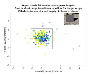
Figure 7: Scatter plots of error in meters with respect to the  $2.3m \times 2.3m$  target. A bounding box indicates the approximate size of the target.
